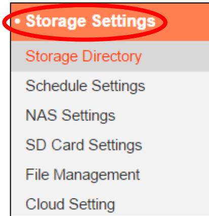
The “Storage Settings” menu enables you to configure the settings for local storage of sound detection events/recordings. You can also configure scheduled recording.
